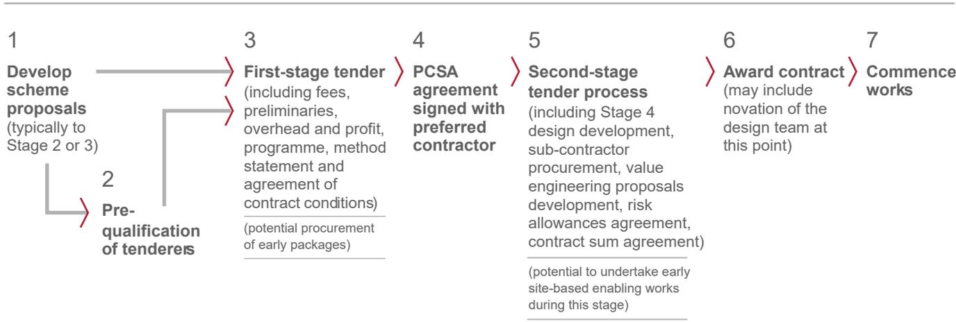
Figure 2: A typical process flow chart for two-stage procurement.
